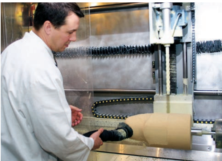
▲ Walter Reed research prosthetist Joe Miller cleans up a foam mold for a prosthetic socket after it was machine carved.
