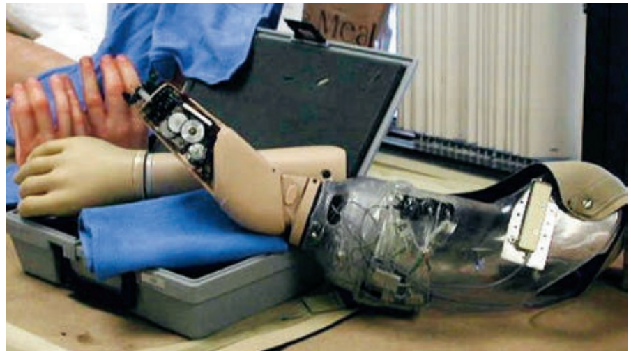
▲ Filled with a variety of innovative electrical components, the myoelectric arm gives wearers a greater range of movement and more comfort.
